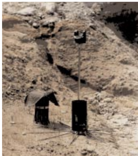
Figure 3-DOD-2. AFW's remote miniature weather station.
