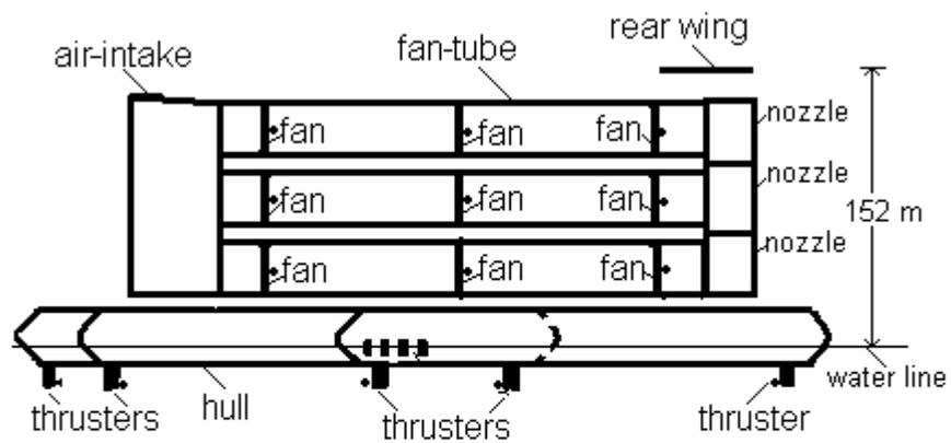
This is a side view of the machine. The machine has fan-tubes, the air-intake is attached to the fan-tubes in the front, and the nozzles in the rear. There are high speed fans in the fan-tubes. The upper part of the machine is supported by the hulls. The rotating thrusters move the machine sideways. There is a rear wing.
