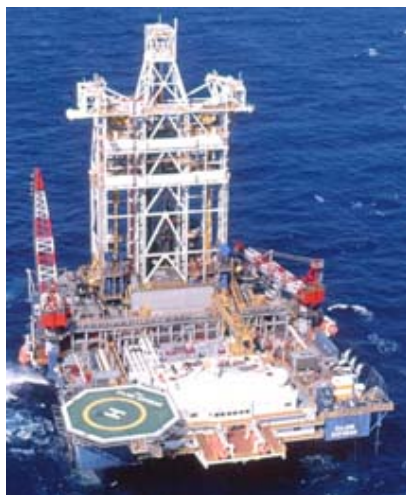
Figure 40: The Cajun Express deep water drilling rig. At 106x70m and with up to 10.6 km (35kft) of pipe down to a pocket of high pressure oil and natural gas, these off shore rigs are analogous to a floating geoengineering platform (Transocean image, http://www.deepwater.com/fw/main/Cajun-Express-52C17.html ).
