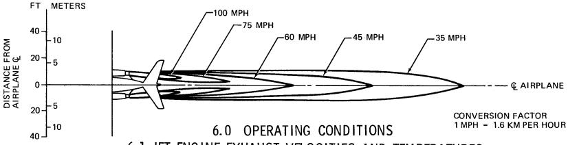
6.1 JET ENGINE EXHAUST VELOCITIES AND TEMPERATURES 6.1.1 JET ENGINE EXHAUST VELOCITY CONTOURS, BREAKAWAY POWER DC-9 MODELS (SERIES 10 THROUGH 50)
