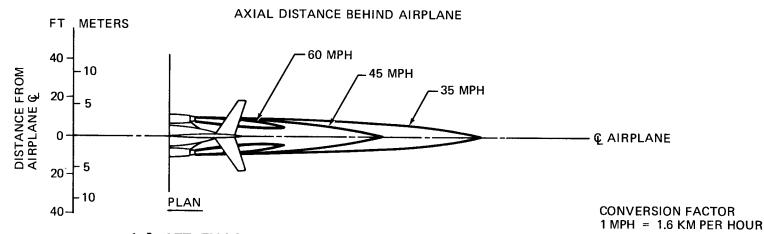
6.1 JET ENGINE VELOCITIES AND TEMPERATURES 6.1.5 JET ENGINE EXHAUST VELOCITY CONTOURS, IDLE POWER DC-9 MODELS (SERIES 10 THROUGH 50)
