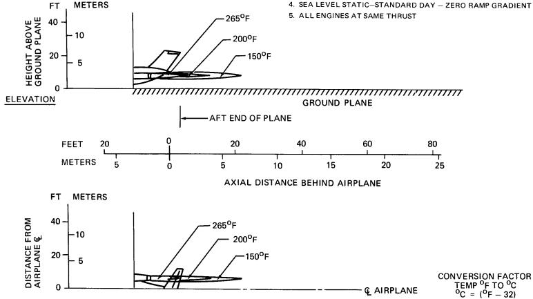
6.1. JET ENGINE VELOCITIES AND TEMPERATURES 6.1.6 JET ENGINE EXHAUST TEMPERATURE CONTOURS, IDLE POWER DC-9 MODELS (SERIES 10 THROUGH 50)
