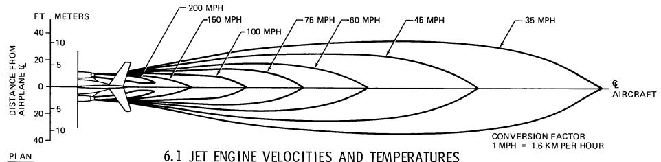
6.1.3 JET ENGINE EXHAUST VELOCITY CONTOURS, TAKEOFF POWER DC-9 MODELS (SERIES 10 THROUGH 50)
